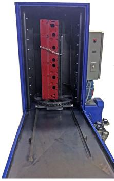
The Terminator SW2444 has a clear 44" vertical height. The 24" diameter turntable supports a 500 pound weight capacity and rolls in and out with minimal effort. Shown with Cummins ISX Cylinder Head
