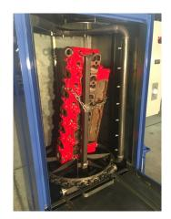
The Terminator **\$W2432** includes a clear 32" vertical height and a 24" rollout diameter turntable. \$W2432 model shown with 5.9L Cummins
