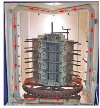
All Axe Equipment water manifolds incorporate Full 360 degree manifold constructed from 2" tubing and designed with radius elbows for high performance water flow. The SW-3660 uses a powerful 15 hp pump pushing 225 gpm at 80 psi through 27 perfectly placed nozzles for fast and efficient cleaning. (Model SW-2832 shown)
