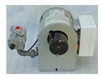
If gas heat is your preference you will like our exclusive state of the art power gas burners. Our power gas burner design puts all the components outside the fire box and away from heat. Components last longer, service is easier and maintenance cost reduced, in addition all sensitive electronics are placed inside a Vapor tight box to eliminate any malfunctions due to moisture.
