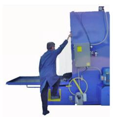
A sturdy footstep and a step assist handle are provided for operator convenience, when loading or unloading, or manual rinsing.
