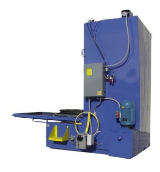
The Intimidator Model is truly intimidating in size and power. Its large 36"x 60" working capacity and 2000 lb weight capacity will accommodate a host of large truck and industrial applications. Standard equipment on the Intimidator features pneumatic door clamps, built in hot tank, manual rollout wheel, and a powerful 15 hp pump motor flowing 225 gallons per minute of hot cleaning solutions for fast and efficient cleaning.
