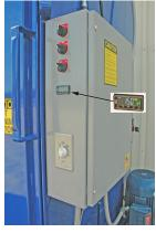
Heat is very important in the cleaning process and that is why every AXE Equipment washer is outfitted with a digital temperature controller for controlling and monitoring the heat process in the tank.
