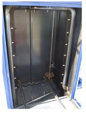
A well designed spray manifold is a key component for good cleaning. The Blue Max series uses large 2" diameter tubing with smooth radius style elbows in a 360 degree design inside the spray chamber for a non restrictive flow. Couple this design with its 5 hp pump and you get 80 gallons of hot water every minute over the parts inside with 50 psi of pressure for quickly sheering away grease and grime.
