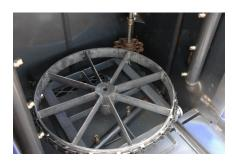
Gear driven turntable with spring loaded safety clutch guarantees consistent turntable rotation within the spraychamber for a complete cleaning job.
